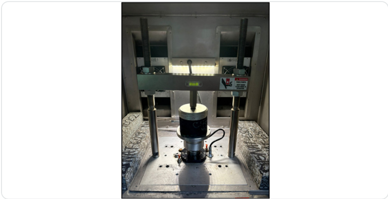
Figure 2: (a) ITS Test, (b) Dynamic Creep Test.
