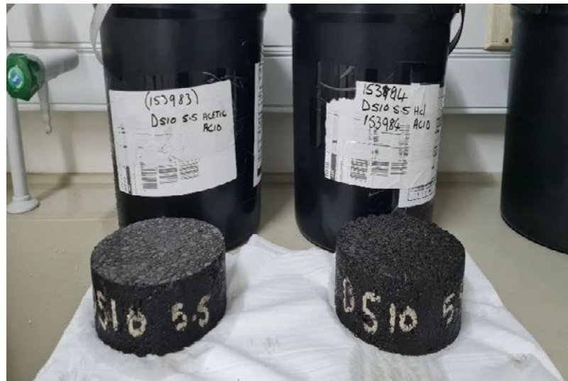
Leachate test samples: coal waste briquettes (right) vs. conventional (left)
