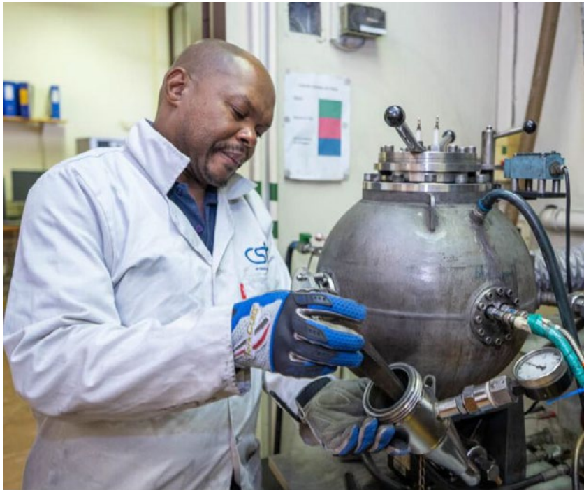
20-litre explosion vessel being charged with a coal dust sample
