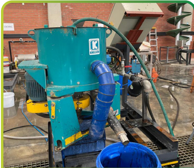
Figure 1: Keelson CVD6 pilot scale setup
