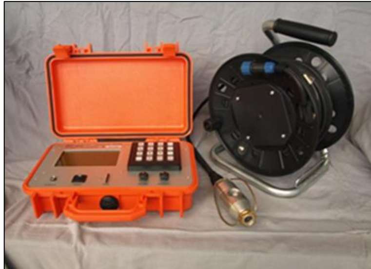
Figure 29: Blast Hole Temperature Logger Mk8 USB ( Insight Technical Support, 2021 )
