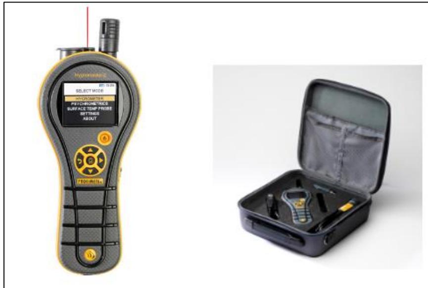
Figure 14: Hand-held Thermo-Hygrometer ( Laboratory Equipment Supplies, 2021 )
