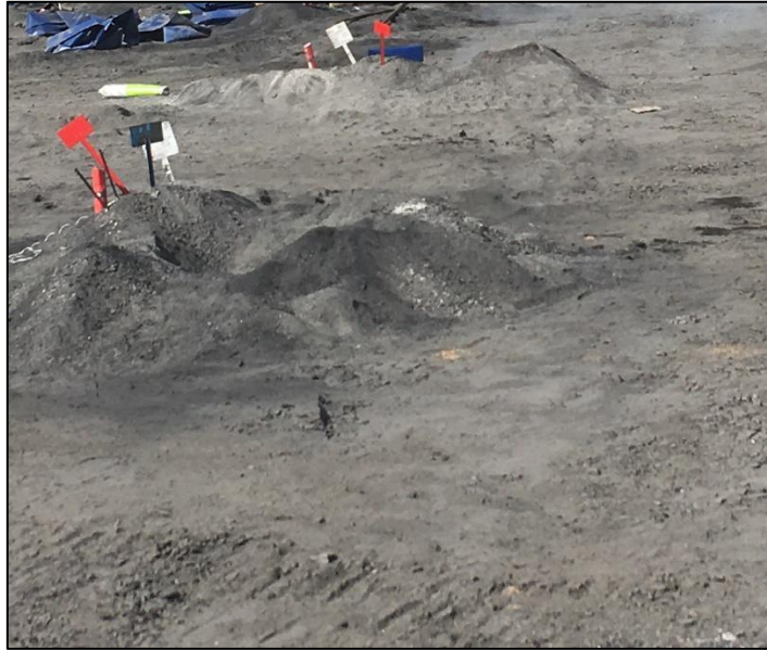
Figure 36: Drill holes with red tags (>55°C) and white tags with hole information captured
