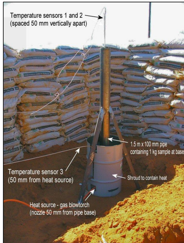
Figure 6. Set up for the tests on bulk emulsion-based explosives (Rorke & Conradie, 2018)
