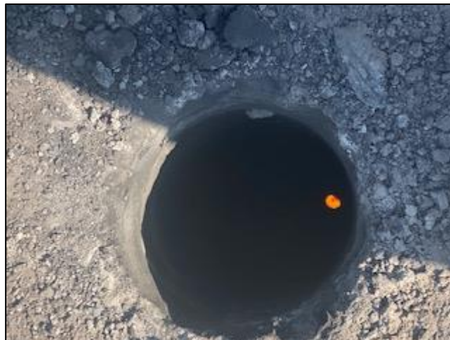
Figure 39: Fire observed in a hot hole on a block at Mine A
