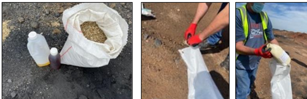
Figure 62. A set up of the Serviplex foam plug before it is inserted into a test hole
