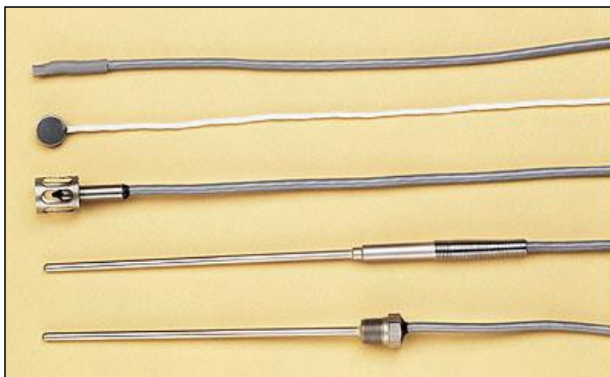
Figure 12. Examples of thermistor-based temperature probes (Missouri S&T, 2021)
