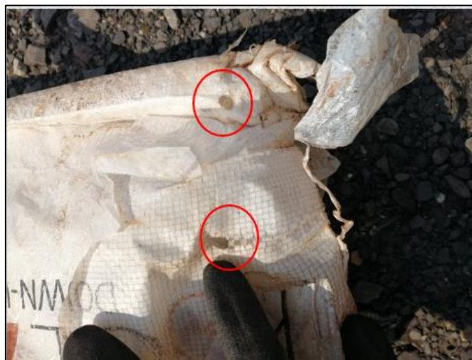
Figure 59. A puncture gas bag after retrieval from the test hole
