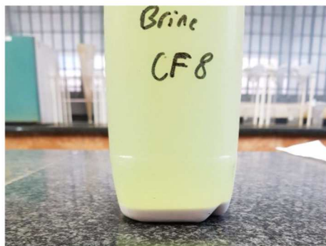
a) Precipitated salts observed before brine has cooled down completely
