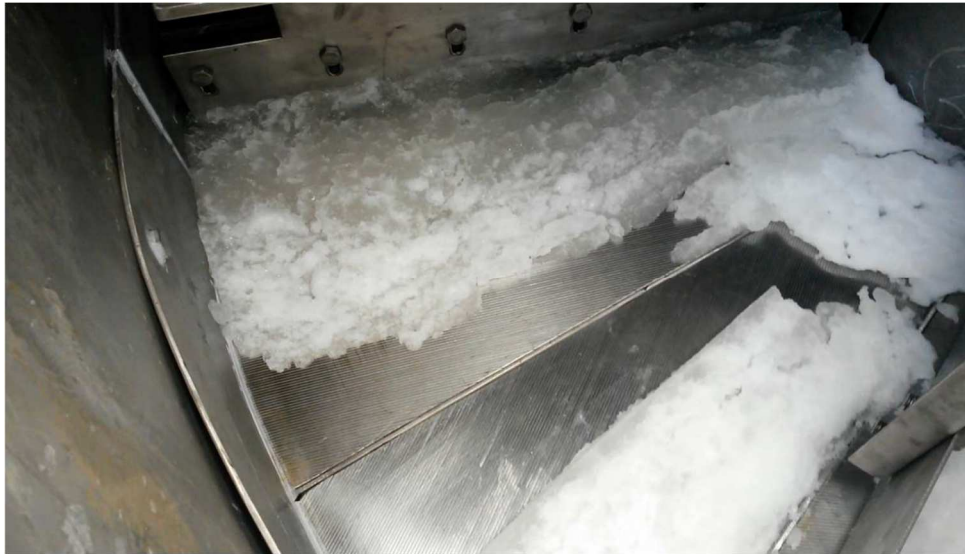
Figure 3.7: First ice production with new ice removal and dewatering equipment
