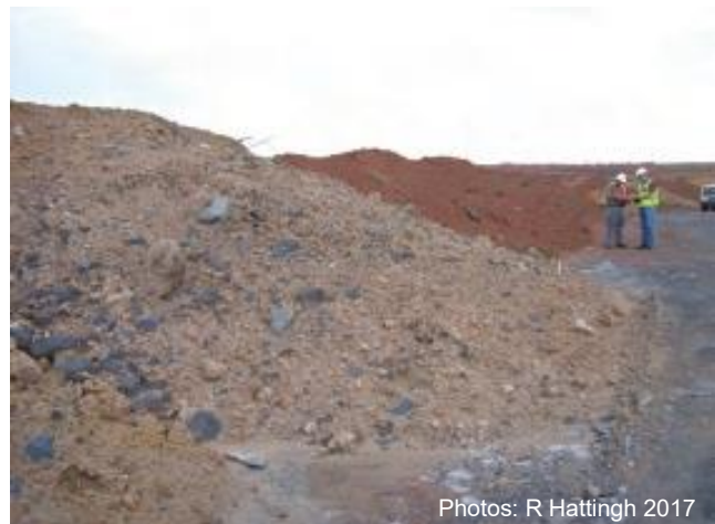
Soil contaminated by fly-rock
