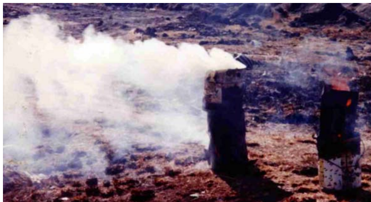
Figure 3: Visible effects of an old and a new way of burning coal in a coal stove. Source: Attie van Niekerk, NOVA Corporation.
