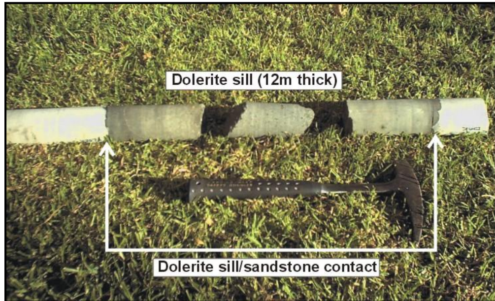
Figure 4.1: Photograph showing the very sharp and smooth contacts between a 12m thick dolerite sill and the sandstone host rock.
