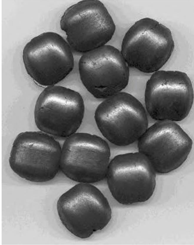
**Figure 2: Devolatilised binderless briquettes produced from the 1 ton/h Zemag Roll Press 400 x 140**
