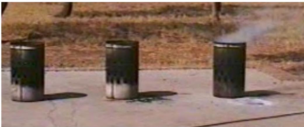
**Figure 4: Combustion tests: Comparison of devolatilised binderless briquettes, raw binderless briquettes and D-grade sized coal (photo taken 50 minutes after the fire had started)**
