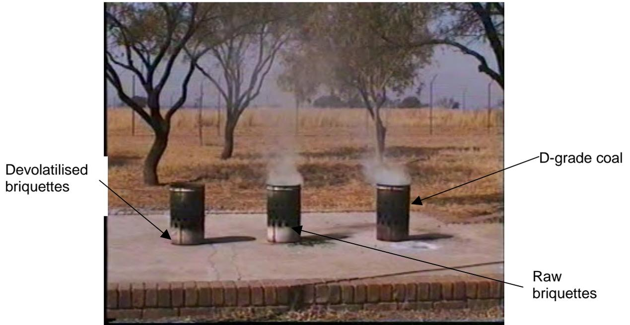
**Figure 3: Combustion tests: Comparison of devolatilised binderless briquettes, raw binderless briquettes and D-grade sized coal (photo taken 30 minutes after the fire had started)**
