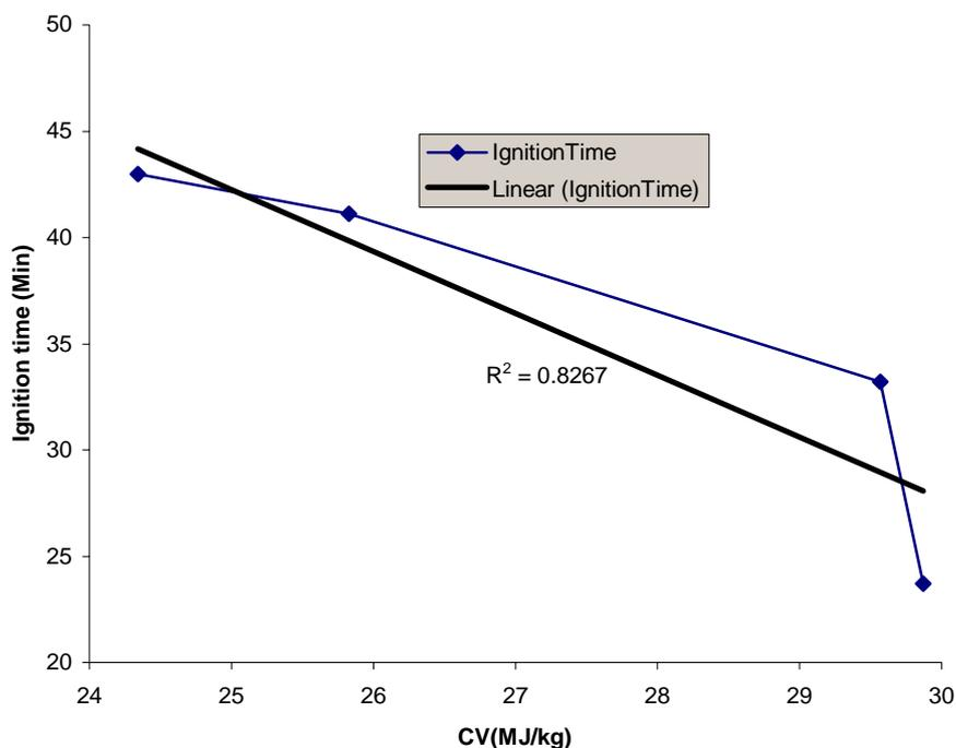
**Figure 7: Correlation between CV of the fuel and ignition time**
