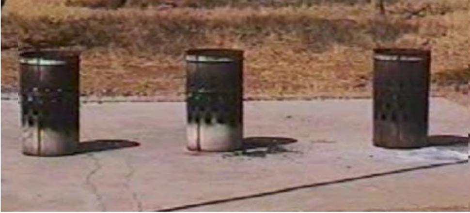
**Figure 5: Combustion tests: Comparison of devolatilised binderless briquettes, raw binderless briquettes and D-grade sized coal (photo taken 75 minutes after the fire had started)**
