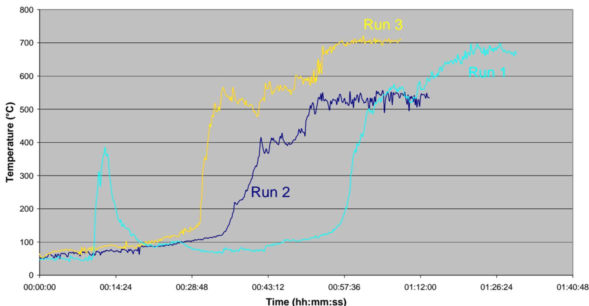
**Figure 6: Temperature profile of the KK devolatilised binderless briquettes produced from the demonstration plant**
