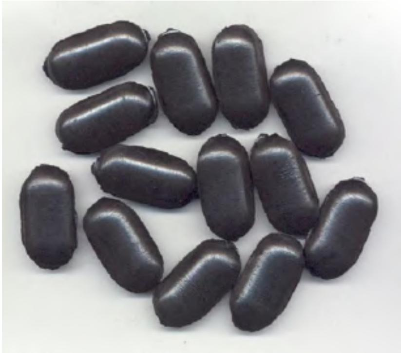
**Figure 1: Binderless briquettes produced from the laboratory press (Komarek B100)**
