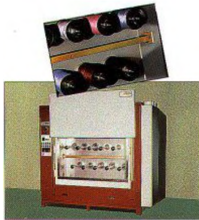
Figure 14: Microwave dryer for textile reels
