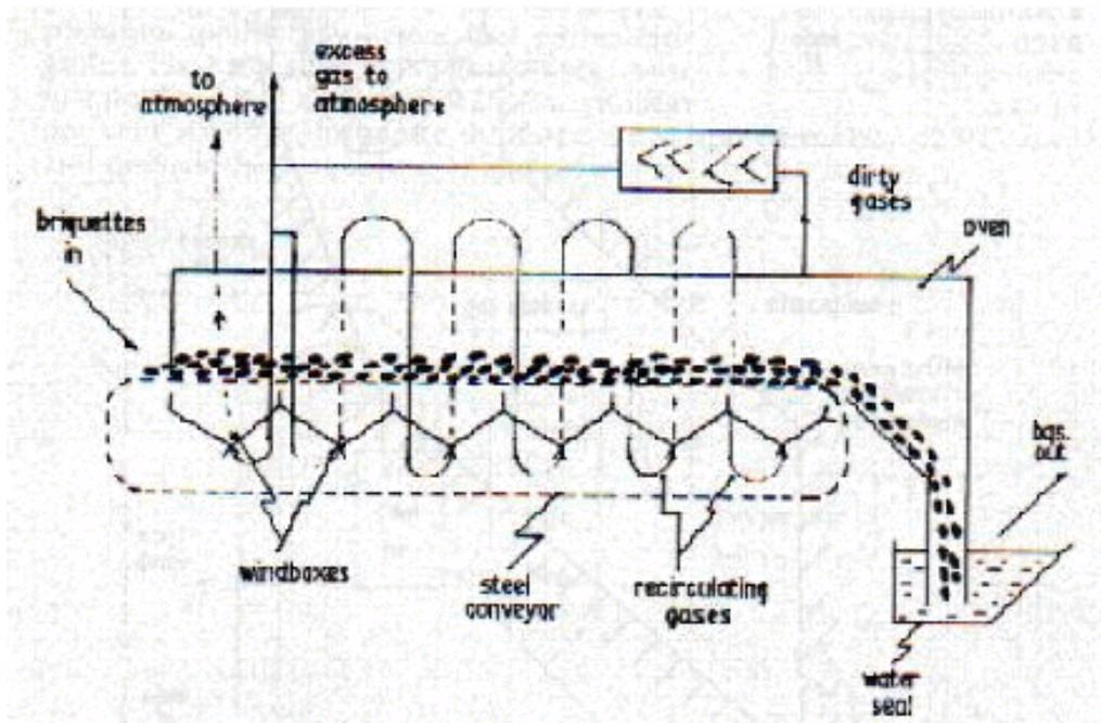
Figure 7 - Oxidising Curing Oven
