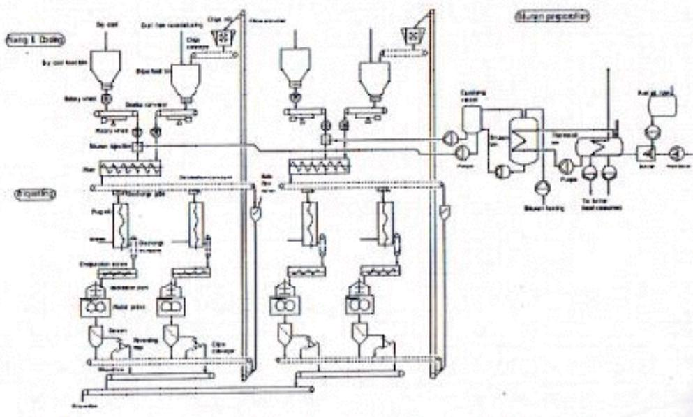
Figure 2 Typical Flowsheet - Briquetting with a Binder
