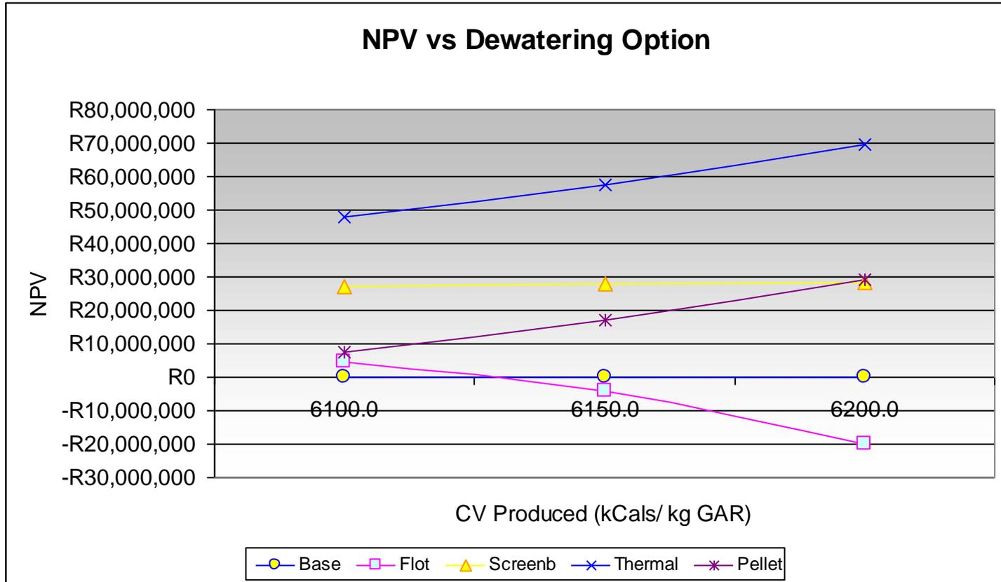
When the capital cost of equipment is taken into account it can be seen that thermal drying is still the best option but that pelletising gives a lower return than the screenbowl centrifuge until a product of 6200kcal/kg is produced. However a positive return is achieved at all levels and the improved handling characteristics of the product makes the agglomeration process worthy of consideration.
