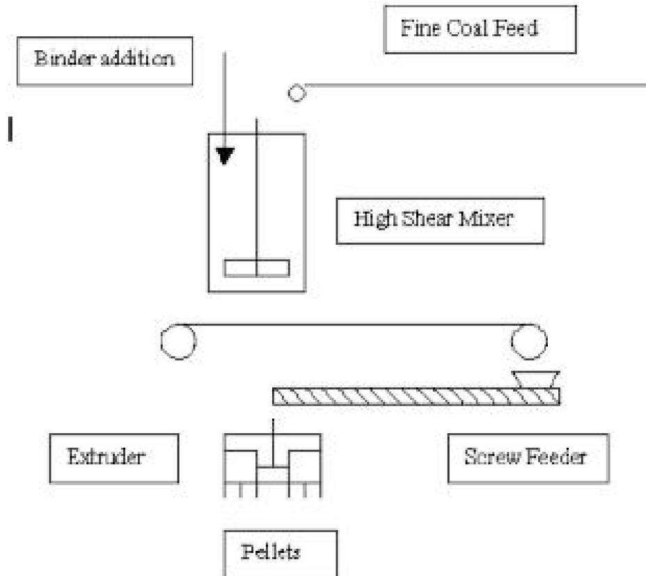
Figure 9 - Flowsheet for Extrusion Pelletising
