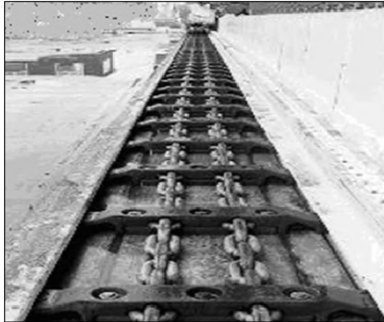
Figure 5-2: Armoured Face Conveyor (courtesy of JOY Mining Machinery)
