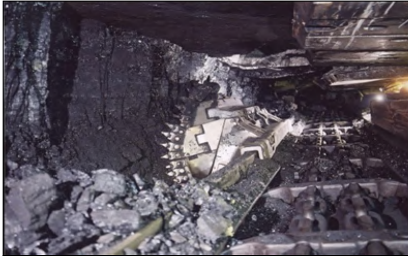
Figure 3-2: The automated plow system (courtesy of DBT)
