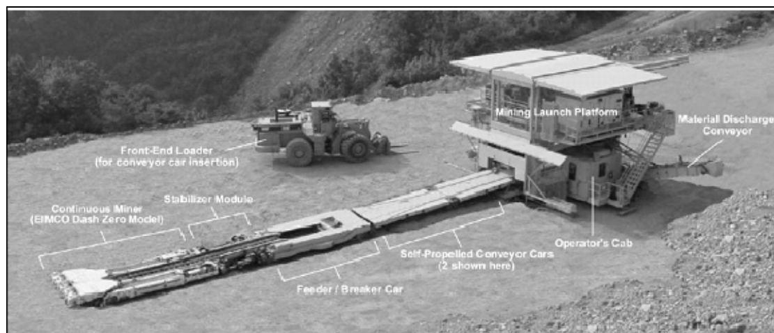
Figure 6-3: The complete NEXGEN system layout (courtesy of NEXGEN Highwall Mining Systems)
