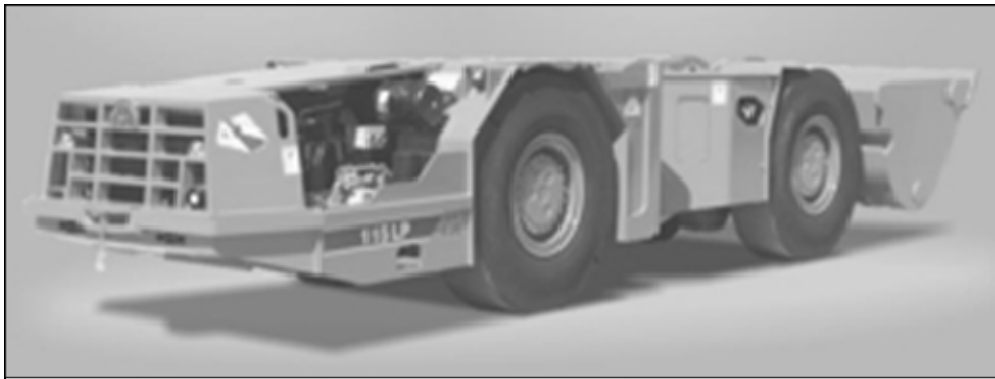
Figure 8-4: The EJC low profile LHD (courtesy of EJC Mining Equipment Inc.)
