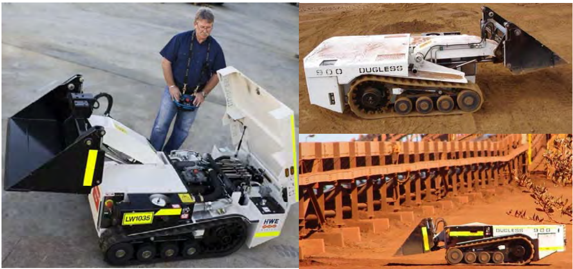
Figure 12: Douglass 900 – diesel powered
