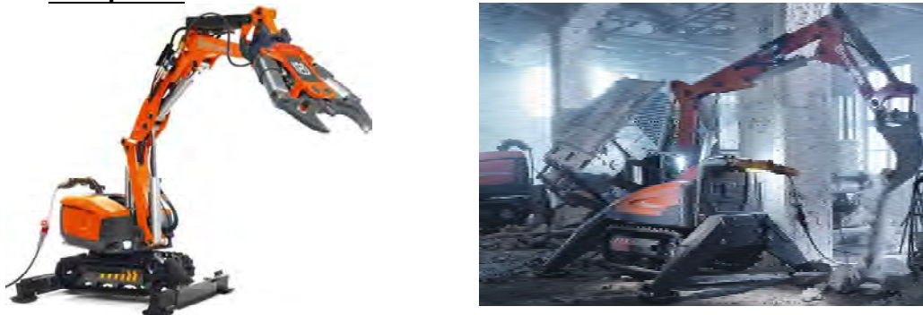
Figure 10: Husqvarna DXR 140 – electrical tether powered
