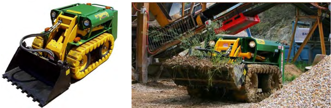
Figure 11: Kanga D800R – diesel powered
