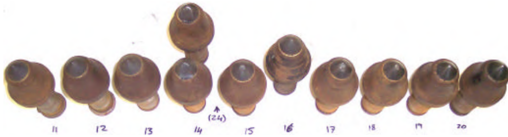
Figure 7: Full spiral of picks removed after cutting sump
