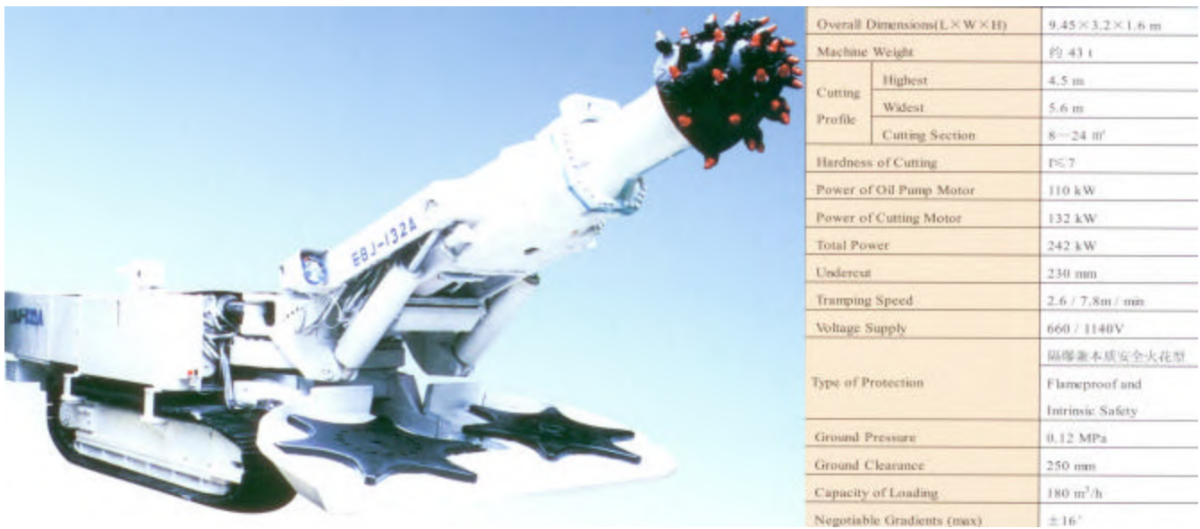
Figure 10: Specifications for EBJ-132 Tunnelling Roadheader
