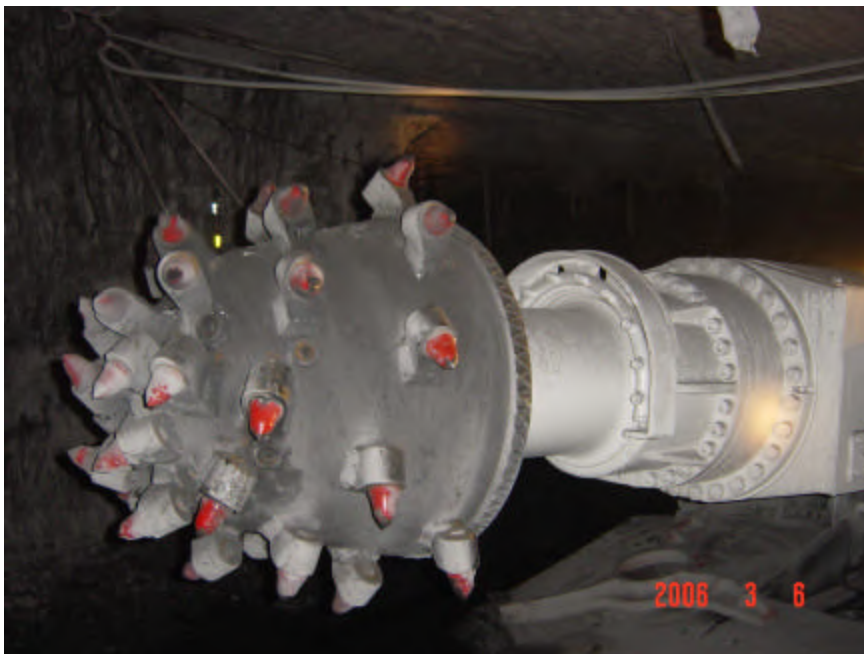
Figure 4: The business end of the Vibrant Roadheader – the cutting head
